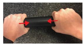
Gripping the tube, Push the corrugated joints together as shown.
